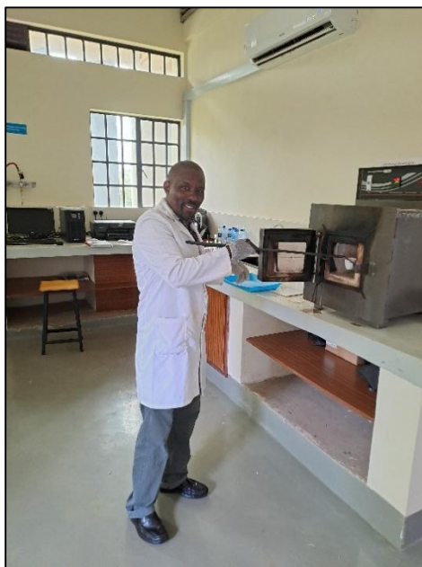
Figure 3.3: Calcination of the \text{Fe}(\text{OH})_3 to form Maghemite ( \gamma\text{Fe}_2\text{O}_3 )
