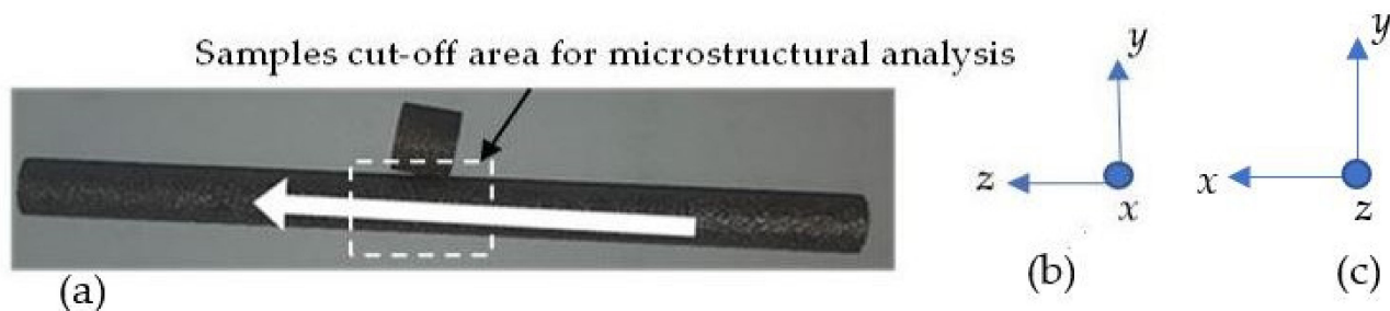
Figure 1. (a) A typical fabricated cylindrical rod of DMLS Ti6Al4V(ELI) that was then cut up into cylinders of 6 mm height for microstructural analysis and further tests. In (a), the white arrow shows the build orientation, (b) the EOSINT M280 machine standard co-ordinate system and (c) the coordinate system of the SEM used for this study with reference to the orientation of samples.
