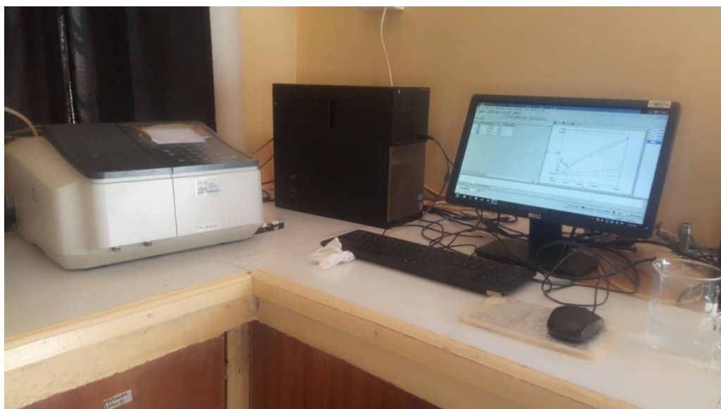
Figure 3.4: UV-1800 Shimadzu UV Spectrophotometer (UV-Vis) at Chuka University
