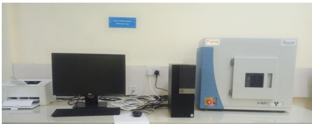
Figure 3.1: ARL Equinox 100 X-Ray Diffractometer (XRD) at Murang'a University of Technology
