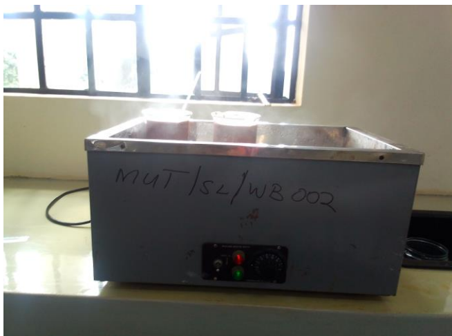
Figure 3.4 Heating of cassava peels containing pearl millet amylase enzyme extract in a water bath
