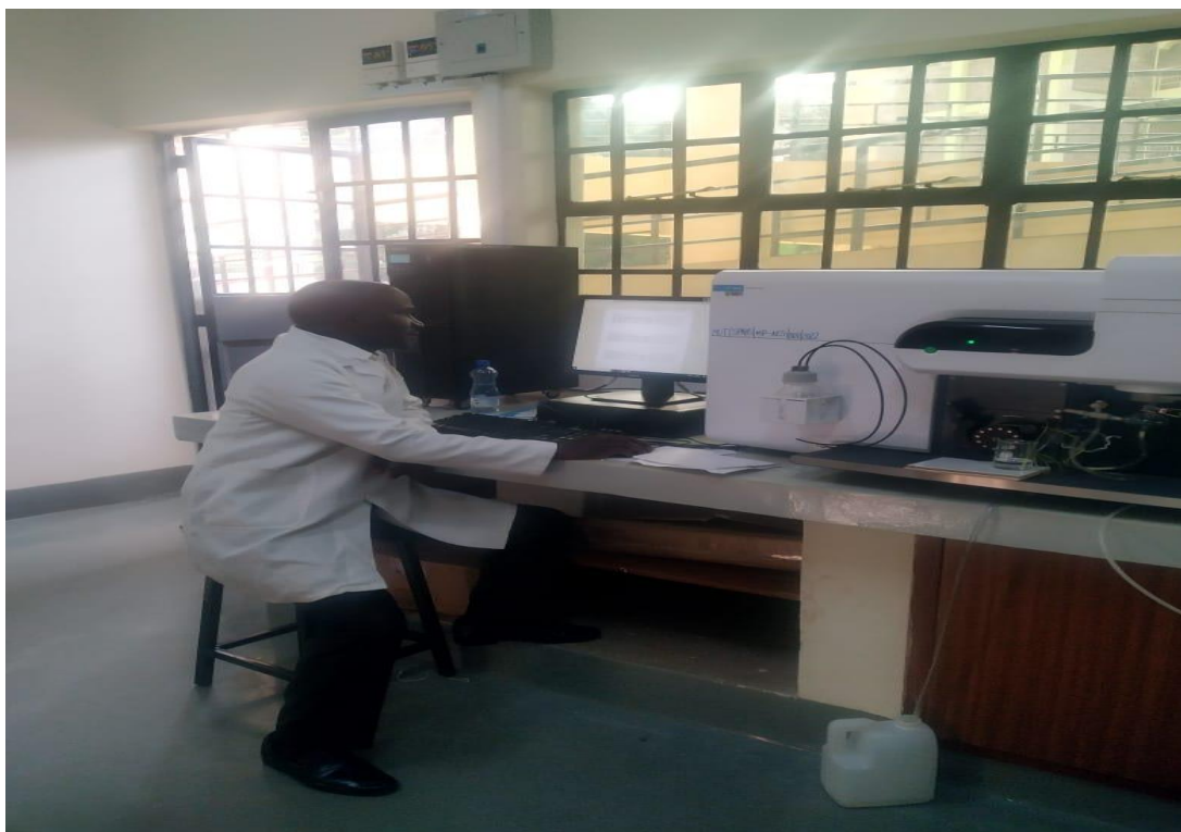
(a) Elemental Analysis using MP-AES Instrument
