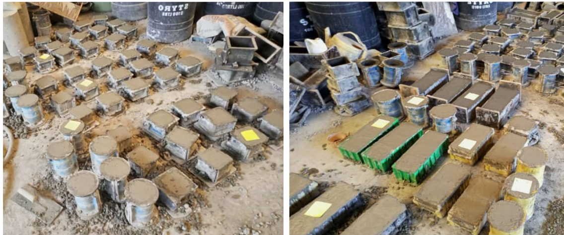
FIGURE 4 | Cast test sample with Ronier fiber integrated.
