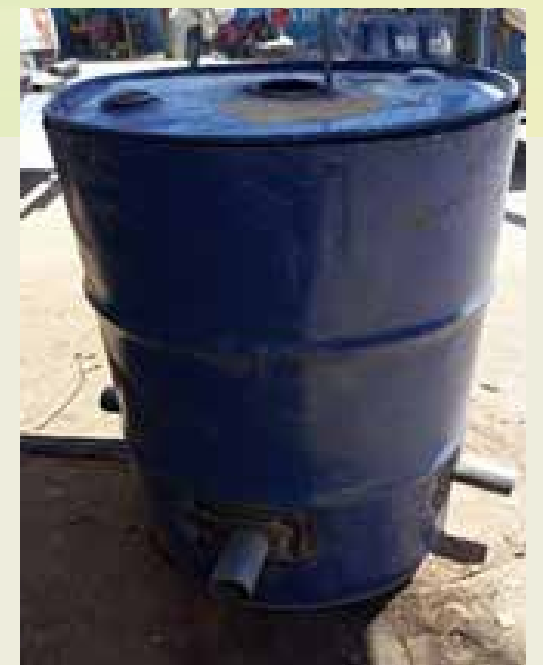
Drum fabricated into a kiln for Charcoal production
