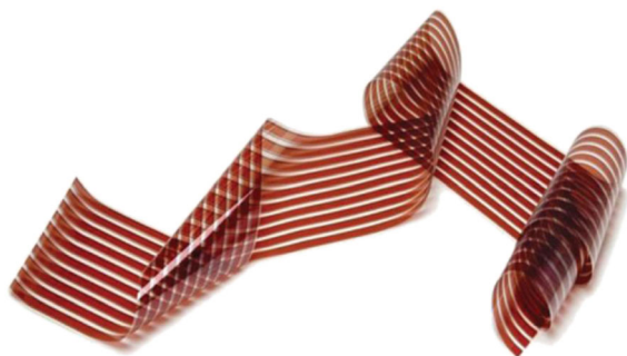
Figure 2. Organic solar cell cast on a flexible substrate. It can be stretched, rolled or even curved in any direction [30].
