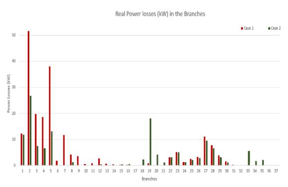
Fig. 6. Real power in 33-bus system before and after reconfiguration
