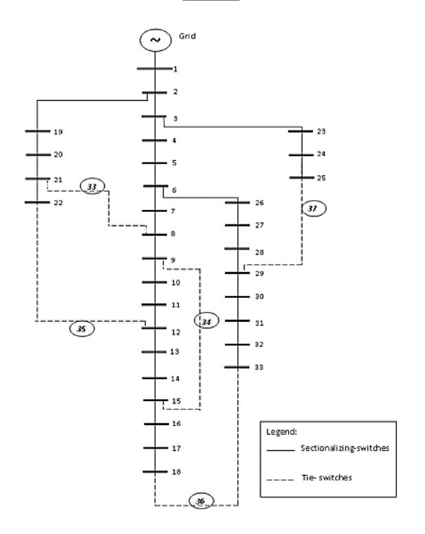
Fig. A1. Single line diagram of IEEE 33-bus RDS
