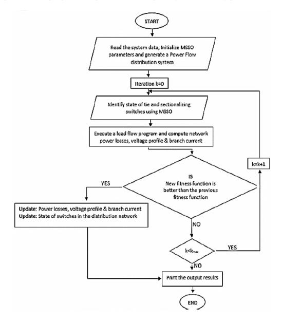
Fig. 4. Flowchart for reconfiguration process
