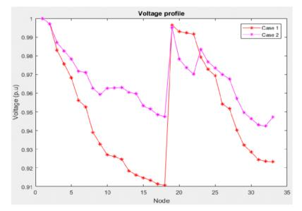
Fig. 5. Voltage profile before and after reconfiguration Case 1 and Case 2
