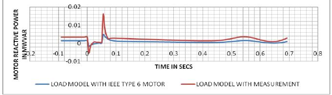
Fig. 3 Industrial reactive load model and load model with measurement
