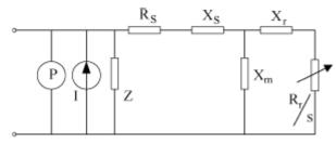
Fig.1. Equivalent circuit of the composite load model
