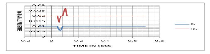
Fig 6 PowerFactory load flow sensitivity of active power with respect to Rr and Rs
