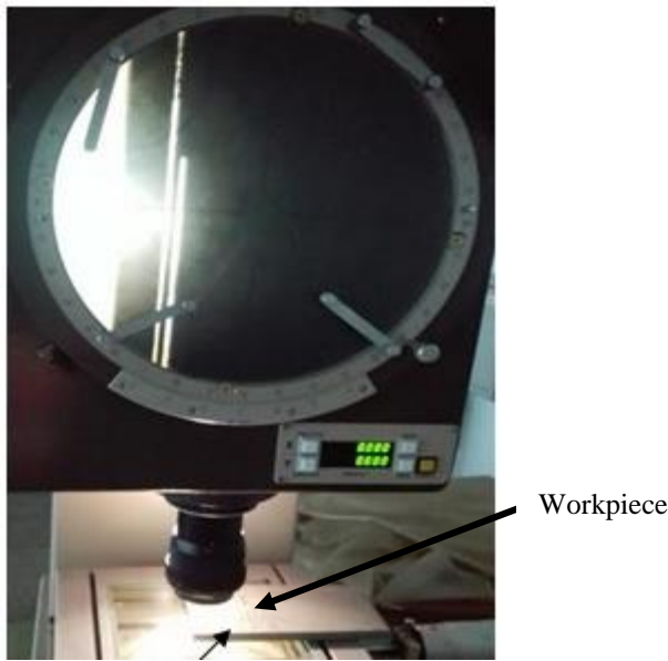
Figure 4: Set up for measurement of gap width using profile projector
