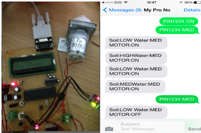
Fig.13: Moisture low motor running at High speed
