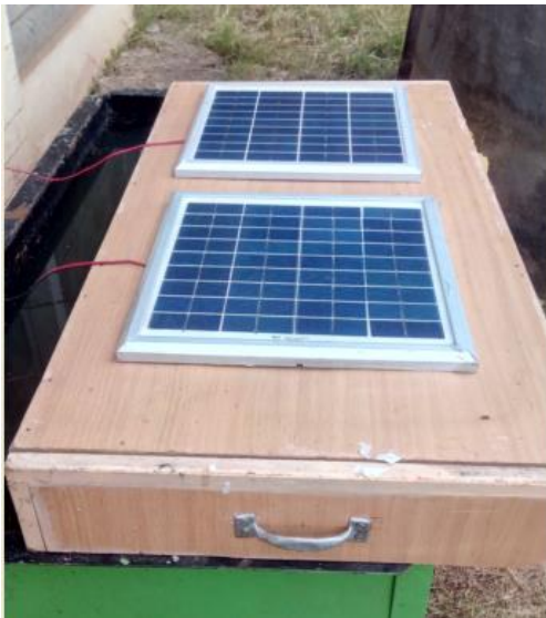
Figure 2: Characterisation of the 13Wp PV Modules
