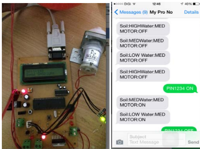
Fig.14: Moisture medium motor running at medium speed
