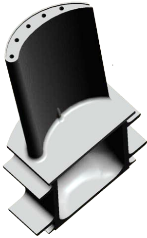
Fig. 3. Turbine blade with cooling Channels
