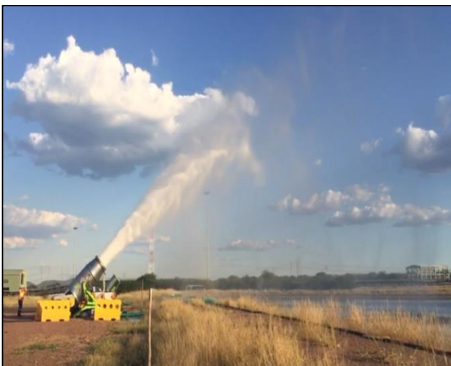
Fig. 1 Mechanical evaporator equipped with a booster pump
