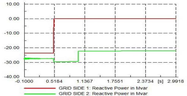
Fig. 21 Reactive power controller.
