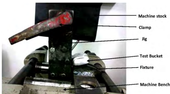
Fig. 4. Set up of the bending experiment
