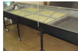
Fig. 3: Tray arrangement in the drying tunnel of the HSBD
