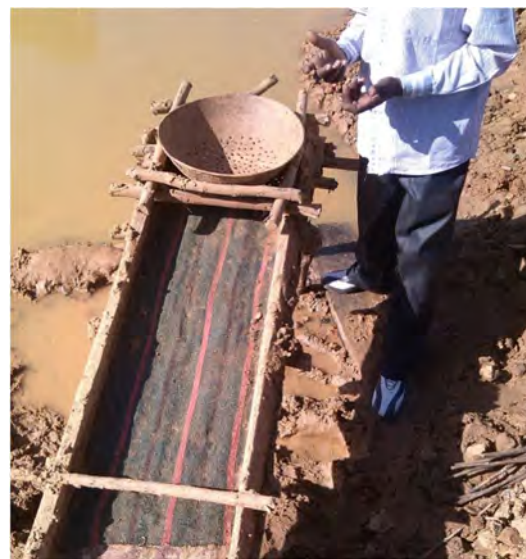
Fig. 1: Sluice used for concentration of gold ore
